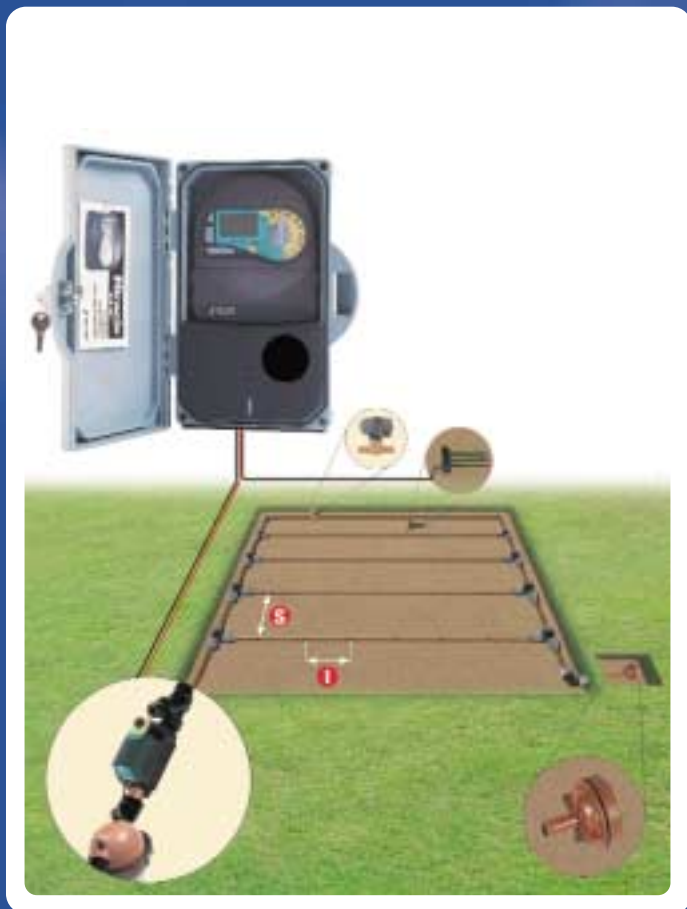
Techline sub-surface grid-layout
