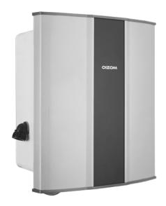
Dustroid® is an Online Particulate Monitoring system to measure the concentration of dust particles in the ambient air. It is capable of monitoring various particulate size ranging from 1 micron to 100 microns such as Ultrafine Suspended Particulate Matter (UFPM), Suspended Particulate Matter (SPM), Respiratory Suspended Particulate Matter (RSPM) and Total Suspended Particulates (TSP). It works on Active Sampling method to count particulate matters using a highly accurate laser beam.
