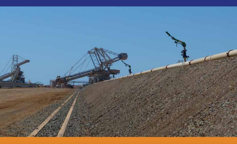
The Stockpile Spray System provides automated water or chemical crusting of stockpiles to prevent dust lift off.
