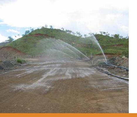
The Haul Road Spray System provides automated, high frequency, light watering of the haul road to prevent dust lift off. It does it without the high labour or equipment costs associated with water tankers.
