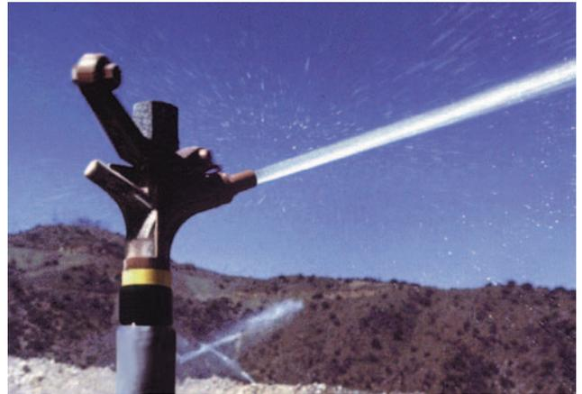
Impact sprinklers that are mounted to a riser should be stabilized to preserve the integrity of the throw. When using risers in gold/silver mining, use carbon steel or stainless steel pipe. When using risers in acid copper leaching, use stainless steel pipe.
