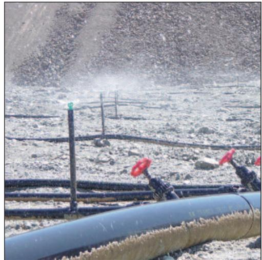
The CMS mini-Wobbler is designed specifically for high sulfuric acid solutions used for copper leaching.
